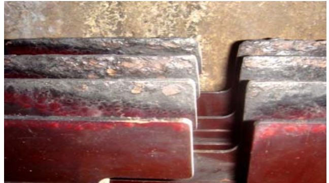
Burn marks on the electrical switch which feeds the current theatre block
